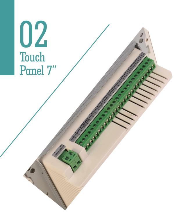
Speaker 30W + Speaker 30W -Speaker 30W + Speaker 30W -Speaker 30W + Speaker 30W -Speaker 30W + Speaker 30W -AUX ROUT AUX GND AUX LOUT Active Subwoofer+ Active Subwoofer -AUX RIN AUX GND AUX LIN Door Bell+ Door Bell -Track Pause + Track Pause -Touch Panel Screen On/Off + Touch Panel Screen On/Off -Touch Panel On/Off + Touch Panel On/Off -Security Alarm Switch + Security Alarm Switch -485 A 485 B 220VAC-N 220VAC-L
